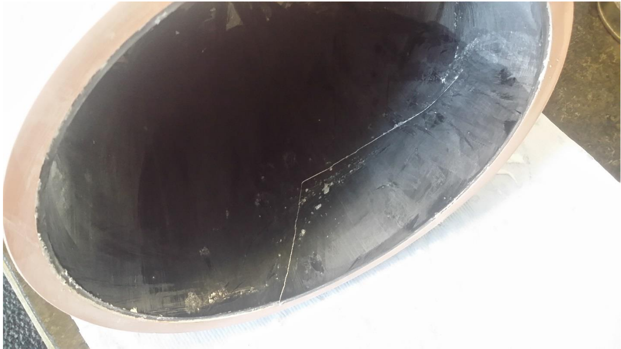
Figure 15: Cracked Stycast after cold-cycling of initial copper bonded absorber
